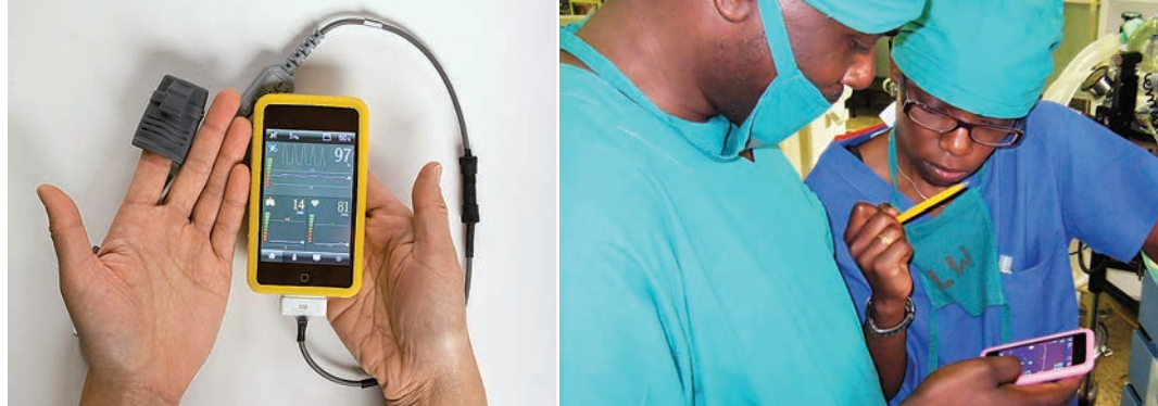
The mobile phone pulse oximeter; health workers in Uganda learn to use the device. PHOTO CREDITS: NATURAL SCIENCES AND ENGINEERING RESEARCH COUNCIL OF CANADA; JACQUI HUDSON.
